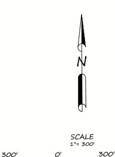
BEARINGS ARE BASED ON NAD83(96) CLEARWATER COUNTY COORDINATE SYSTEM
